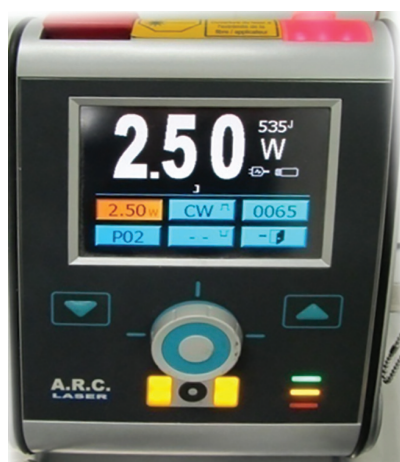
Fig. 3: Diode laser (Fox, ARC, Germany). For lasing the samples of this study, a wavelength of 980 nm and output of 2.5 W was used
