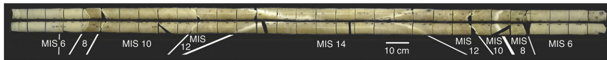
Fig. 3. Core CA recovered from the Texas Toothpick using the drilling system shown in Fig. 2. This image shows the two halves of the core laid flat and thus shows both sides of the core, as the result of the longitudinal sectioning of the core sketched in Part 5 of Fig. 2C. The top of the original core is the horizontal line separating the two halves. The dark vertical lines crossing the core are the cuts made perpendicular to the core, as shown in Part 2 of Fig. 2C. The lower half of the image shows the core from the side, with its top up, whereas the upper half of the image shows the core inverted vertically, as suggested by Part 5 of Fig. 2C. Coring passed from one side of the Texas Toothpick to the other, so that the oldest section of the core is in the middle (MIS 14), and MIS 12, 10, 8 and 6 are represented in both the proximal and distal halves of the core. Note that coring in this manner allows both sides of the stalagmite to be sampled for redundancy.
