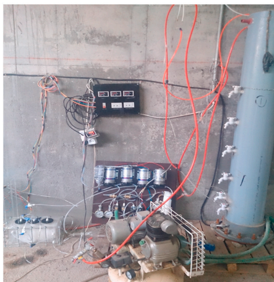
Fig. 1. A) Schematic diagram of IMBAF: (1) Influent reservoir tank; (2) BAF; (3) Air diffuser; (4) Air flow meter; (5) Air compressor; (6) Backwashing water pump; (7) reservoir of BAF effluent; (8) valve; (9) UF pressure pump; (10) Pressure gauge; (11) UF backwashing pump; (12) UF permeate reservoir; (13) RO pressure pump, and B) the actual picture.
